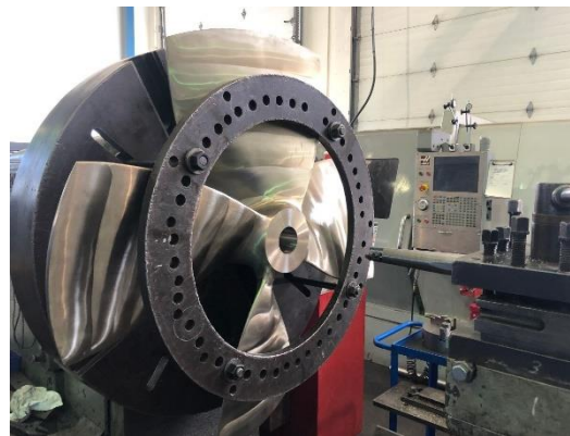
A new 55" Kaplan propeller being machined
