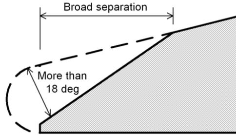
Many sources recommend that the anti-singing edge be applied from the 40% radius (0.4R) fully to the tip, or even slightly beyond [Carlton, 1993]. It has also been noted that erosion of the blade edge is a risk if the new edge were made too thin.
