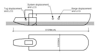
You will want to remember to add appendage drag. (This typically amounts from 5% to 10% of the bare-hull drag.) Also, many ITBs have significant hull and superstructure area, so wind drag may be significant.
