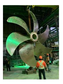
Service Marine also uses TrueProp, which is software for propeller inspection and repair. As HydroComp's partner company, it pairs well with PropExpert. "We use TrueProp on our scanner arm for retro-engineering and pitch adjustment for better geometry," explains Dominique. "We use this to find vibration problems and where we need to fix it."
