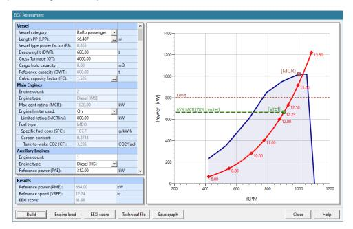
Suitable for virtually all ships under EEXI restriction, the *EEXI Assessment* utility in NavCad Premium provides quick and resource-friendly design guidance when the need comes to investigate where a ship stands regarding EEXI compliance. At the conclusion of the evaluation, the generated report can be used as reference documentation for quality assurance and benchmarking of future EEXI compliance calculations.
